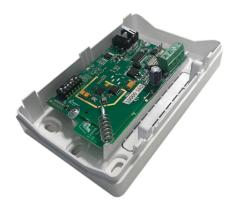
Radio transceiver modules which allow use of the wireless devices listed in Comelit VEDO series control panels. They allow the use of up to 32 sensors, 16 sirens and 32 remote radio controls. Housed in a white flame-resistant plastic container, complete with anti-opening and anti-tear tamper systems that can be isolated. It can also be housed inside containers art. BOXPLASTIC, BOXMETAL and BOXFLUSH. Dimensions (W x H x D)  $126 \times 80 \times 32$  mm.
