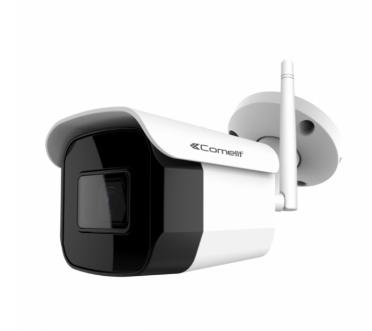
Day & Night colour Wi-Fi IP bullet camera, 3.6 mm fixed lens, FULL-HD resolution (1080p) @15 ips, IP66 waterproof enclosure, 2 infrared lights with a range of 25 metres (Smart IR) for kit art. WIKIT004S02NB. Power supply unit provided.
