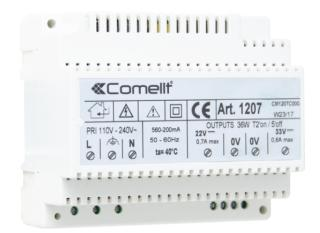
Power supply unit with overload and short circuit protection devices. It has two separate continuous outputs: one to power the external unit and electric lock, and the other to power the monitor. Input voltage 120-230 VAC. Dimensions: 105x85x85 mm (6 DIN modules).
