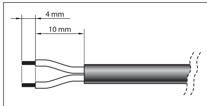
Then proceed with assembly of the **GREY** “L” type socket on the end of the panel cable, as follows:
