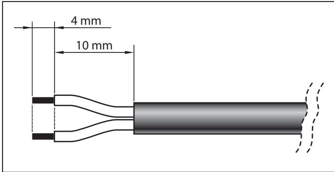
Then proceed with assembly of the **BLACK** "L" type socket on the end of the power cable, as follows:
