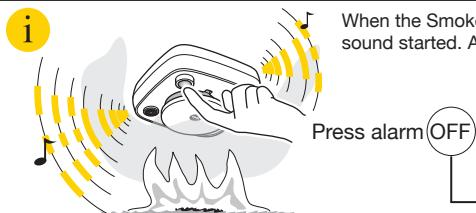
When the Smoke Detector is activated you can silence it 1 minute after the alarm sound started. Active smoke detection will restart after 10 min.
